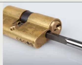
Square cutter used on a lock with a processed stainless steel driver
