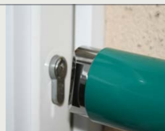
Using the cylinder breaker
