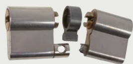
example of a broken reinforced lock using the cylinder breaker
