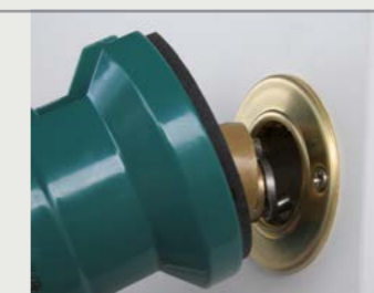
Using the extractor against a bolt barrel
