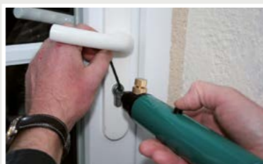
The needle is to be introduced in light contact with the pins
