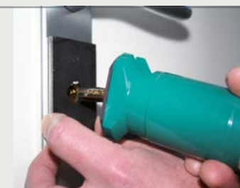
Using the extractor with the back plate against a European lock
