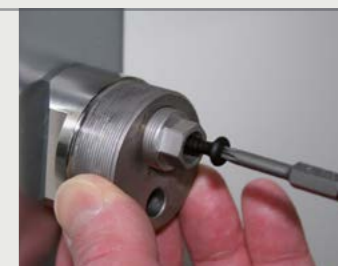
Using the cylinder breaker adaptor
