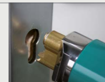
Using the cylinder breaker
