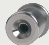
Example of drilling with carbide cutter
