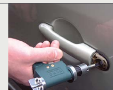
Use of the plug spinner gun to come back to the opening direction
