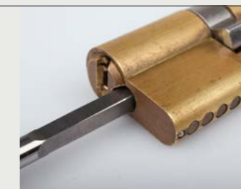
Square cutter used on a lock with front anti-drill insert
