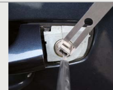
Opening with a pick of a laser key lock on a Golf 6
