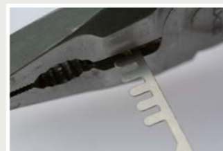
Comb picks to be modified with a sharp pliers according to the wished number of teeth
